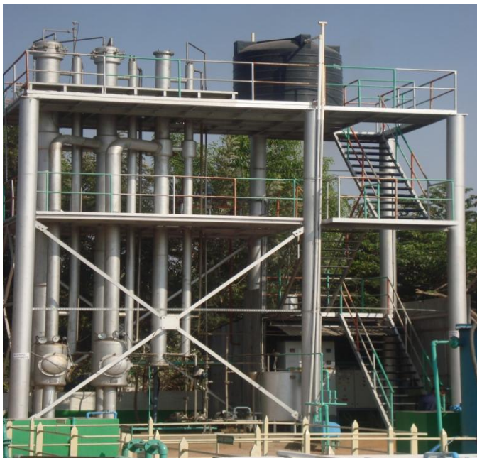
Fig. 12: Three Effect MEE and Recirculation tank which was under back washing process during inspection
