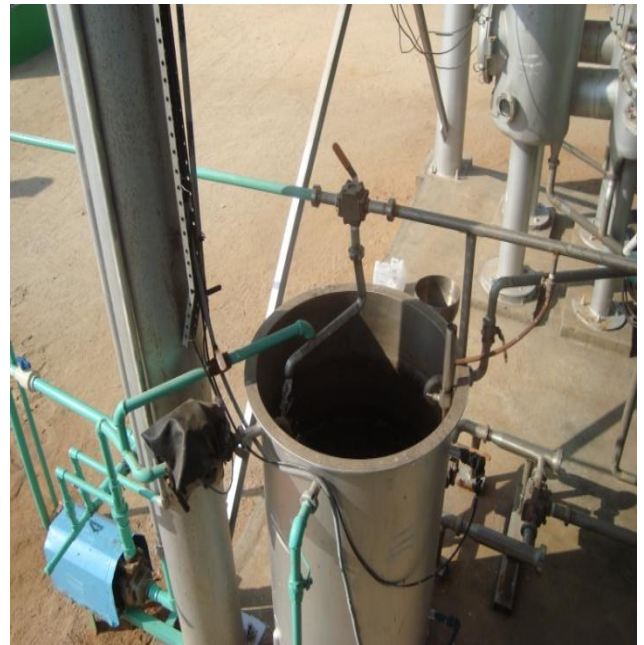
Fig. 12: Three Effect MEE and Recirculation tank which was under back washing process during inspection
